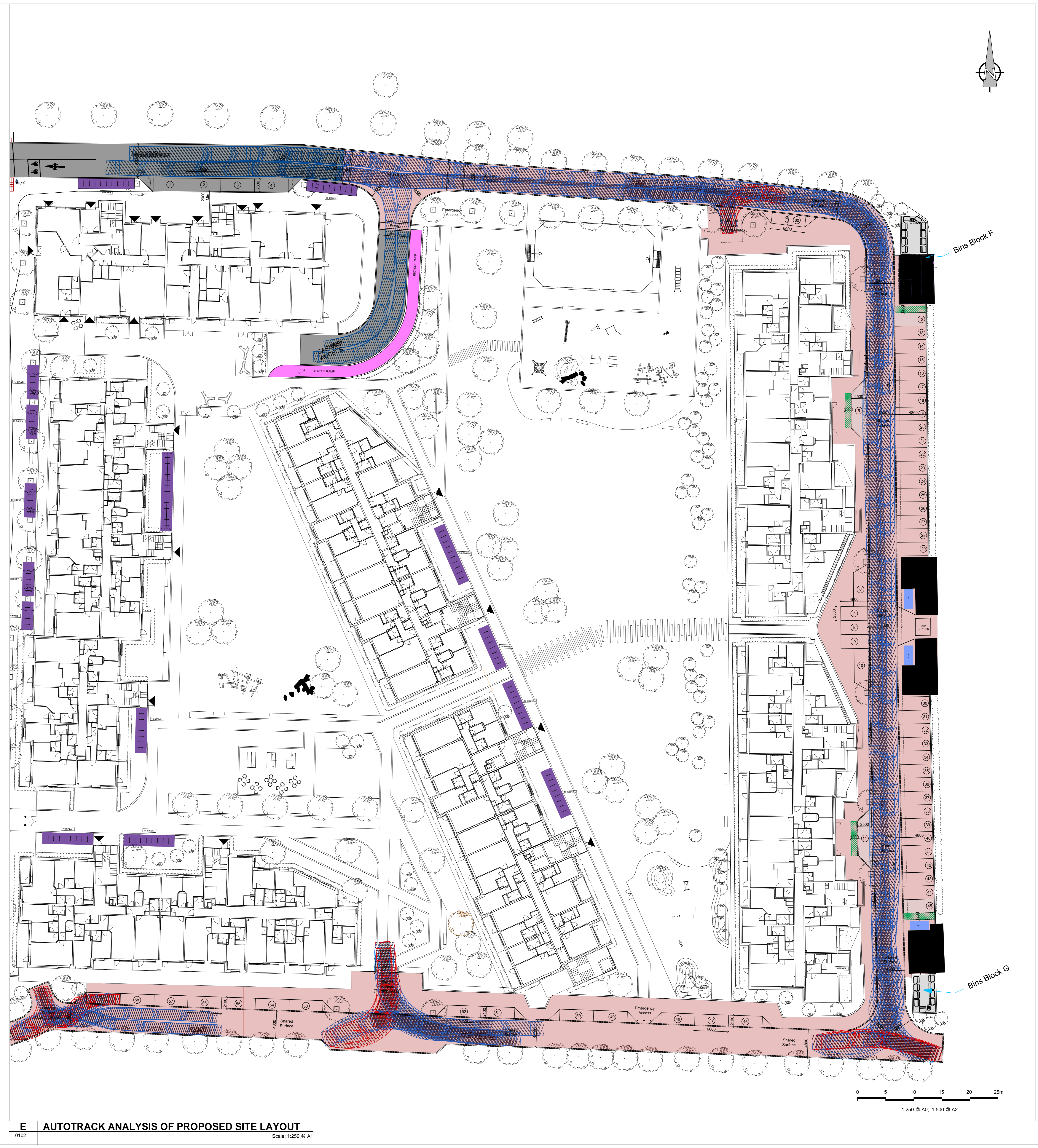
A AUTOTRACK ANALYSIS WITH OF PROPOSED JUNCTION WITH REFUSE VEHICLE Scale: 1:250 @ A1
